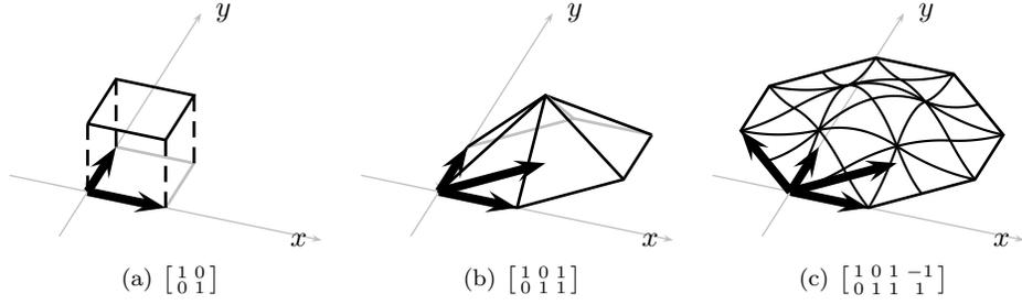
Figure 4. Construction of the ZP-element via directional convolutions.
