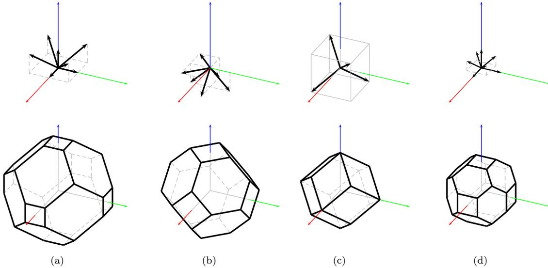
Figure 8. Trivariate symmetric box-splines (top) directions (bottom) supports. (a) 7-direction box-spline on  $\mathbb{Z}^3$  (Section 3.2) (b) 6-direction box-spline on the FCC lattice (Section 5.2 and Section 7.2), (c) 4-direction box-spline on the BCC lattice (Section 6) and (d) 7-direction box-spline on the BCC lattice (Section 8.2).
